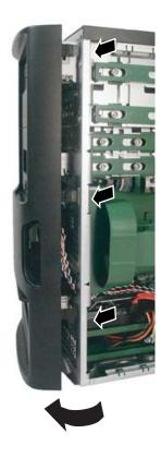
2 Swing the right side of the bezel out to until the left side of the bezel can be disengaged from the left side of the computer, then remove the bezel.
